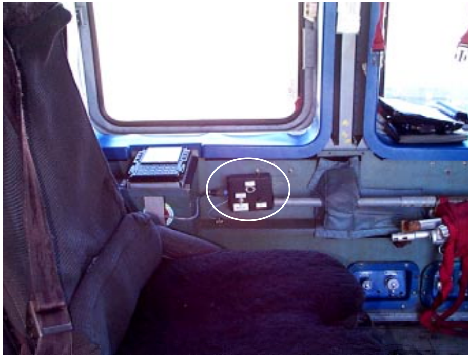
Figure 24. HH-60 Breakout box mounted port side of aircraft
